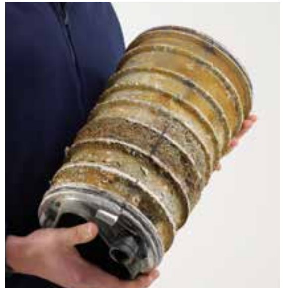
Hard water deposits can block pipe work and damage internal boiler components.
